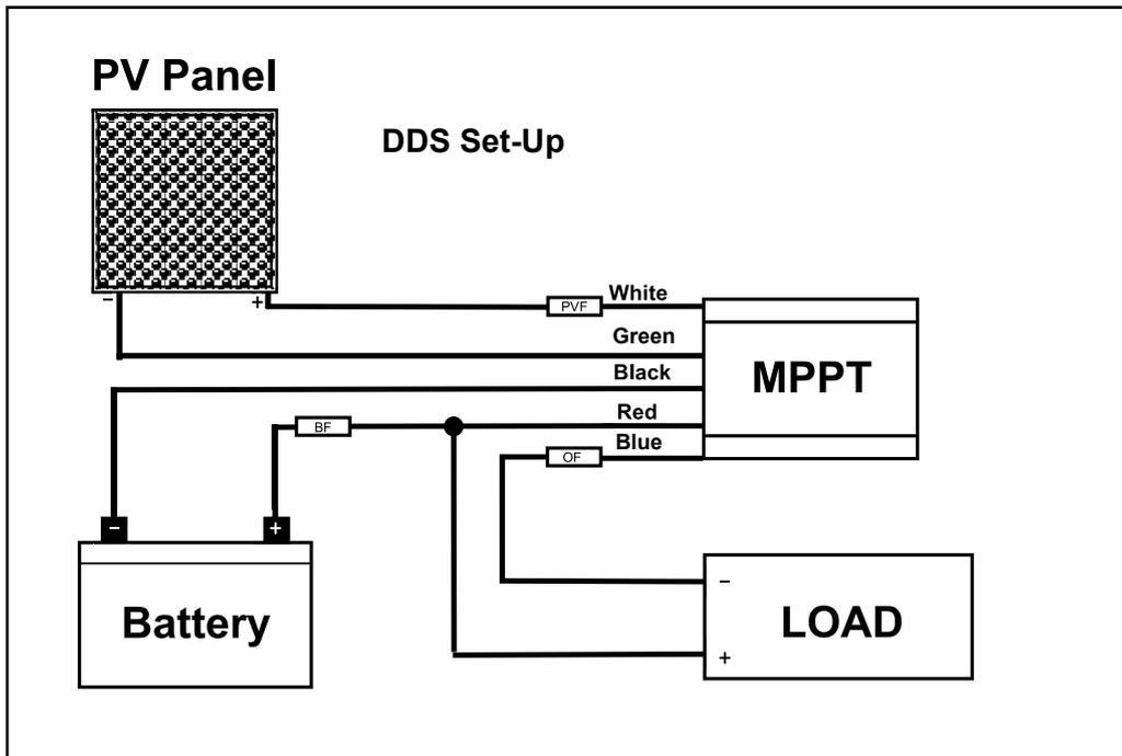
**Wiring With Low Voltage Disconnect :**
