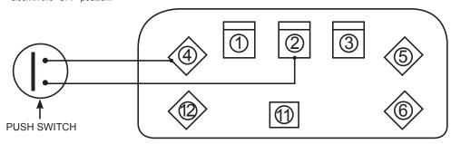
The remote cut off circuit can be connected between terminals 2 & 4.
